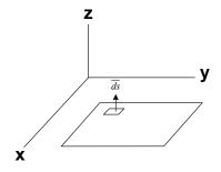
In this example, only the z component of fluid velocity will pass through this surface.
