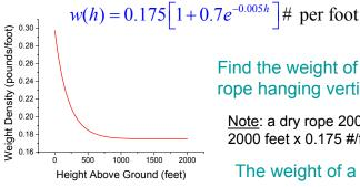
Find the weight of a wet 2000' rope hanging vertically
