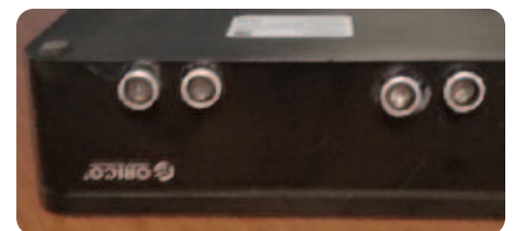
Figure 5: New form factor of the parking sensor as deployed in Parking Lot A
