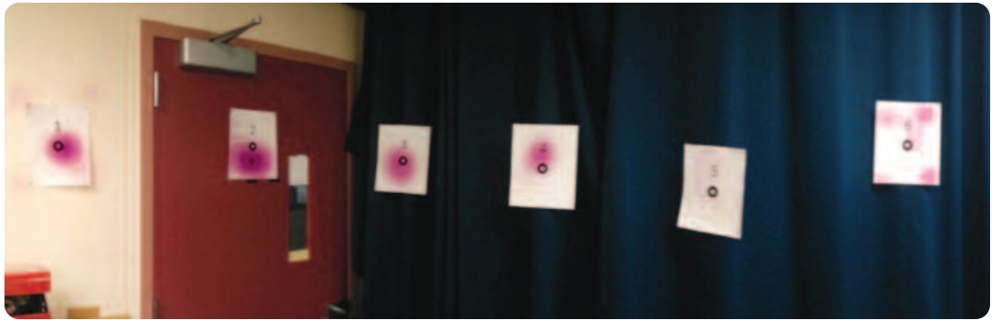
Figure 14: Head-tracking data from HoloLens was integrated with gaze direction data from a wearable eye tracker. This figure demonstrates that this data can be used to accurately measure gaze location in the real world for users wearing HoloLens.
