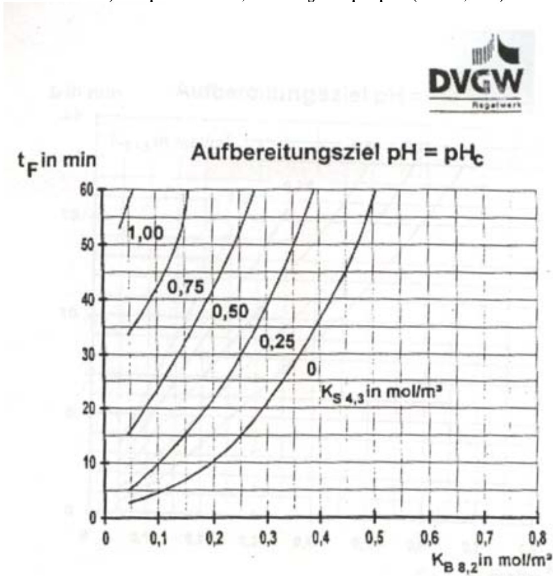
Figure 5. Contact Time as a function of Base Consumption ( K_{B,8.2} ) and Acid Consumption ( K_{S,4.3} ) for Dense Calcium Carbonate (Grain Size 1.0-2.0 mm). Temperature: 10°C, Processing Goal pH=pH c . (DVGW, 1998)
